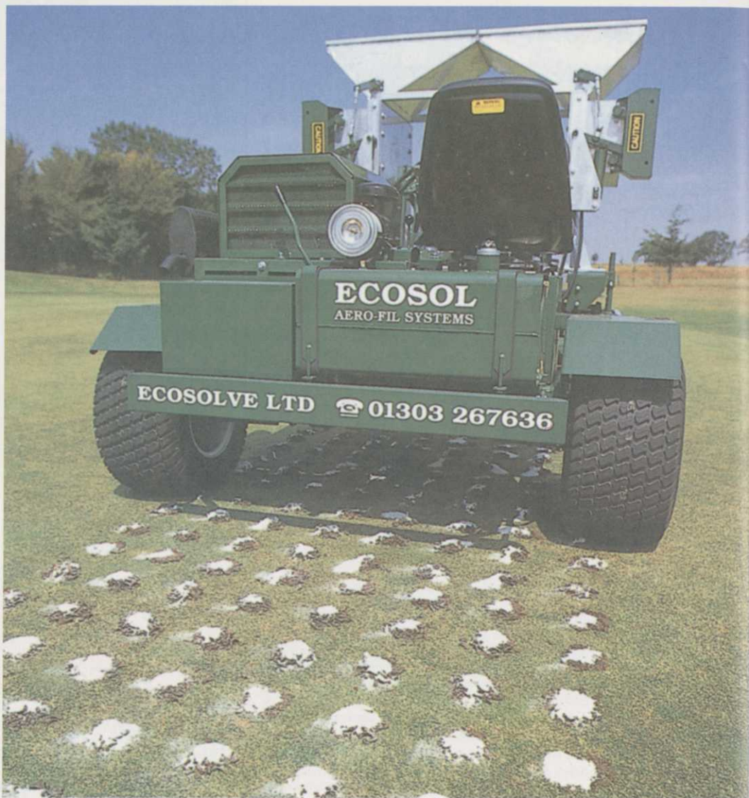
The Show saw the launch of the Ecosol Aero-Fil System from Ecosolve Ltd. The drill and fill aerator is designed to relieve compaction instantly, penetrate the hardest soils, backfill accurately up to 30cm, improve water infiltration, increase root depth and is gentle on the turf which enables play to resume immediately. Launched at the same time vs Ecosol Sportslite, a zeolite soil amendment designed to be used with the Ecosol Aero-fil system's drill and fill.
