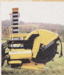
The optional soil clear-up system folds up for easy transport.
