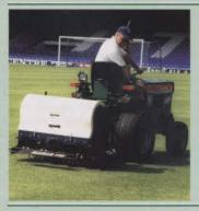
Available in three working widths, able to carry out highly effective turf aeration to a maximum depth of 125mm (5in).
