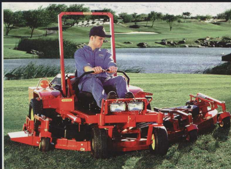
Powerful 38hp diesel 96" cut. Height of cut from seat.
