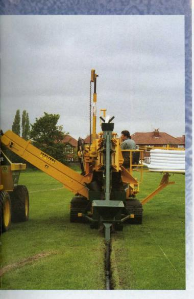
used mainly to augment piped drainage are 'slitting' and 'sand banding'. Such methods are ideal to remove water from specific spots, furthermore they can be used to intercept water, such as from a spring, and channel it to a drain.
