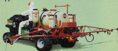
AM-PS Eagle High specification sprayer. Tank sizes 300/600/800 litres. Fitting kits available for all turf utility vehicles.
