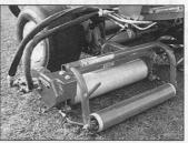
Green speeds can thus be increased without the need to reduce mowing heights. This saves stress on the turf and produces lusher greens, hence the rollers popularity for tournament preparation.
