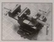
the quick and easy drilling of multiple holes in the workplace without the need to continually remove and adjust the position of the work.
