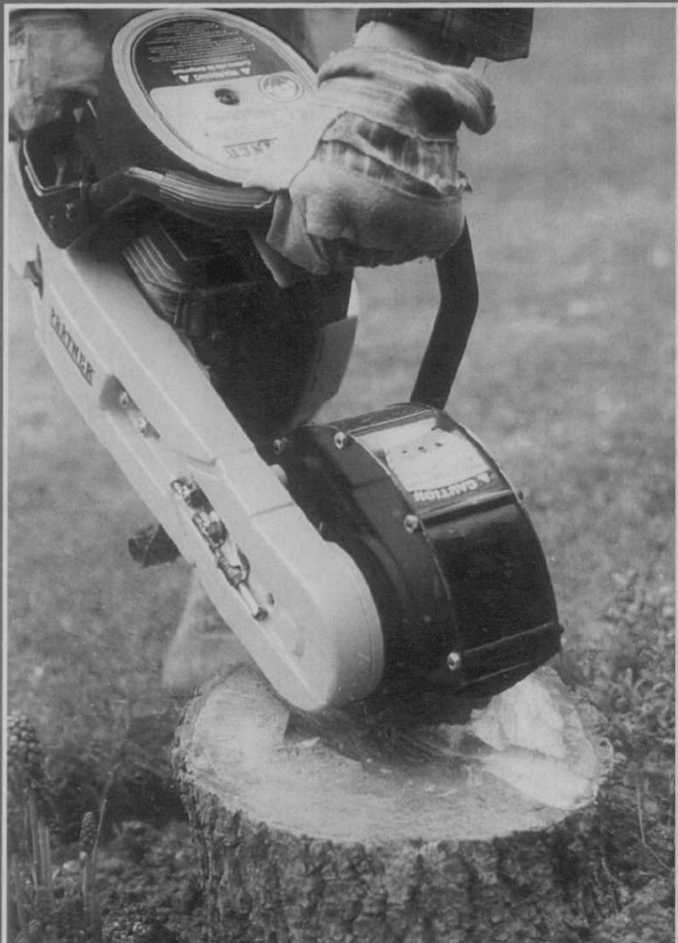
Tree stumps are easily removed with either a hand-held or pedestrian operated stump grinder
