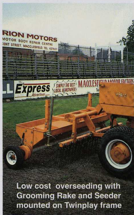
Specially cast, spiral, studded roller creates ideal growing environment for simultaneously broadcast seed.
