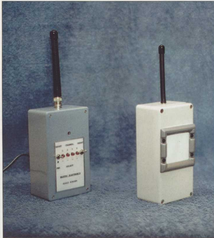
Radio security: A standard four channel portable received and an external detector, with a range of 35 metres
