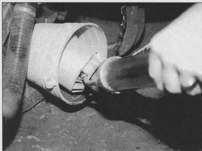
Power take-off guards should be in place, in good condition and regularly maintained. Ensure that their restraining chains are securely fastened in work
