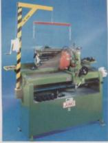
accommodate every make and type of professional cutting cylinder and bedknife. Can 'in-situ' grind many greensmower reels. Water cooled (eliminates dust and heat), simple and fast to use, accurate 'relief angle' grinder.
