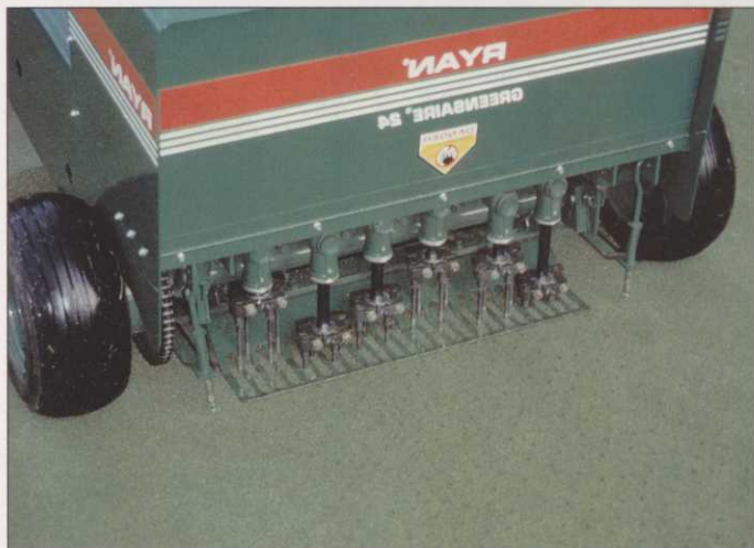
Solid tining has a similar aerating effect to slitting but the round hole holds its shape better in dry weather
