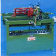
Juno 36". Will accommodate every make and type of professional cutting cylinder and bedknife. Can 'in-situ' grind many greensmower reels. Water cooled (eliminates dust and heat), simple and fast to use, accurate 'relief angle' grinder.
