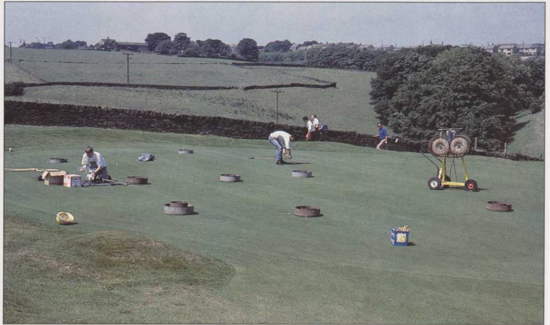
Survey work in action with the concentric rings being used for infiltration measurements
