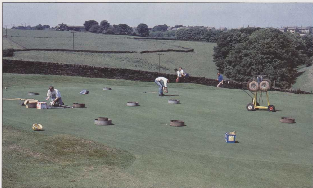
Survey work in action with the concentric rings being used for infiltration measurements
