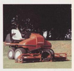
hood assembly which folds back smoothly and the rear cutting unit which slides back to allow total access and ease of maintenance. There is also a major upgrading of the hydraulic drive system incorporating heavy duty wheel motors and automatic 3WD which cuts in when mowing and out when downhill. Power steering is standard and the new Tri-King is available for five or 10 blade reels with a seven blade unit sheduled for introduction later this year.
