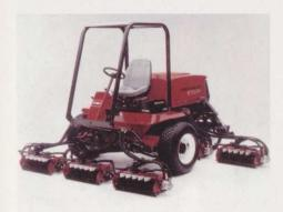
A feature of the new mower is Toro's new L-I-N-K-S cutting unit suspension system which allows the cutting units to hug the turf and reduce bobbing.
