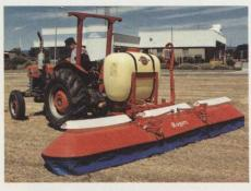
Hardi International launched a new range of Hardi-Rogers Windfoil Boom assemblies to suit de-mount, mounted or trailed Hardi Amenity sprayers. The 4.5 metre boom is available in two versions the full hydraulic folding version which is ideal for large golf course complexes or the budget model with manual fold normally sold to traditional golf courses or local authorities.
