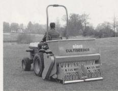
The new SISIS Cultiseeder, a pto driven disc seeder with a working width of 1.2 m was launched at the Show.
