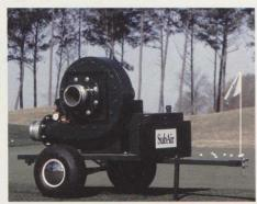
A new American-designed machine which claims to double your green's root mass made its UK debut at BTME 96. **SubAir** was developed by American Golf Course Superintendent Marsh Benson and features a blower which spreads air into the integral drainage system below the root zone of a USGA spec green. This oxygenates the root zone to increase root zone vigour and transfers water vapour to the root zone from the perched water table.
