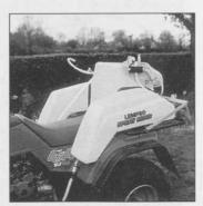
able for spraying widths from one to four metres. An additional feature of the SR10OP is the re-circulation of chemicals achieved through the pressure regulator which provides some agitation.
