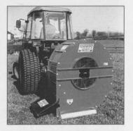
Supported by two heightadjustable castor wheels, the Tornado TM360 XL can be set to produce an air blast up to 128mm (5in) above the ground to suit the depth and quantity of debris to be moved. Twin skids are welded to the base of the fan housing and there is an antiscalp roller to prevent scuffing over uneven surfaces.
