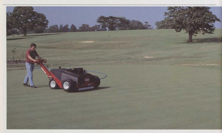
The finest of turfs - that's what this greenkeeper achieves with Toro's unique water injection HydroJect aerator. Able to tackle very wet or rock hard ground conditions, it allows play to resume immediately. On the golf green, bowling green, cricket wicket or tennis court, HydroJect complements conventional aeration methods. And for large turf areas, Toro's Fairway and HC4000 heavy duty aerators cover up to 1.5 acres per hour with ease.
