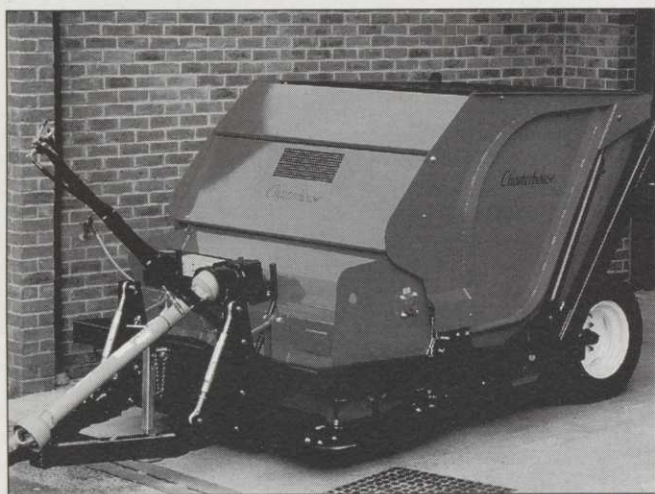
Charterhouse launched its new Turf Tidy which de-thatches dead and deteriorating turf, helps to bring new life to soil and grass while thatch clippings and sweepings are hoovered up into its 2.5 cubic metre hopper.
