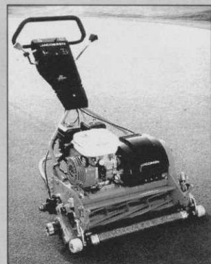
The new 422 Greens King pedestrian mower from Jacobsen complies with the latest EC regulations and is fitted with Operator Presence Controls (OPC). It also has a 22in cutting width and a high-speed 11-knife cutting cylinder. It is powered by a quiet 4hp, four-cycle OHV engine and, with its 11.5in rollerbase, follows contours without scalping. The reel, roller and traction drum are all the same width.
