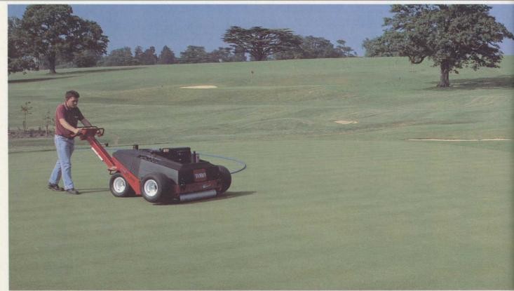
The finest of turfs - that's what this greenkeeper achieves with Toro's unique water injection HydroJect aerator. Able to tackle very wet or rock hard ground conditions, it allows play to resume immediately. On the golf green, bowling green, cricket wicket or tennis court, HydroJect complements conventional aeration methods. And for large turf areas, Toro's Fairway and HC4000 heavy duty aerators cover up to 1.5 acres per hour with ease.
