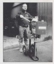
years" but only bought its own (second hand) machine last year. The Fuji Robin Dagger soil ameliorator, to give the full name, is a unique machine with a single tine, this is driven into the soil by vibration from the two stroke engine when a charge of compressed air is released to lift and shatter the soil from the tip of the tine. The machine is self con-
