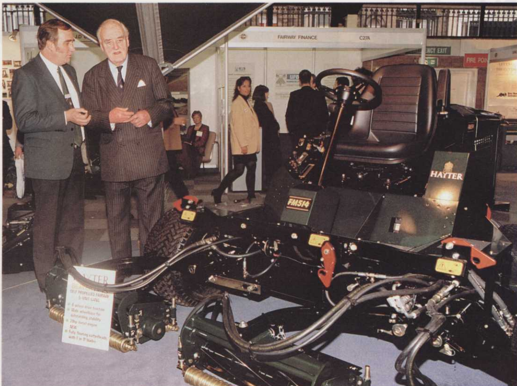
Lord Whitelaw admires the Beaver FM 514 fairway mower. Features include newly designed 26in fully floating cutterheads which are available with 7 or 11 blade cutting reels offering a clip rate of 131 or 206 per metre. Power is provided by a 29hp Lombardini diesel engine.
