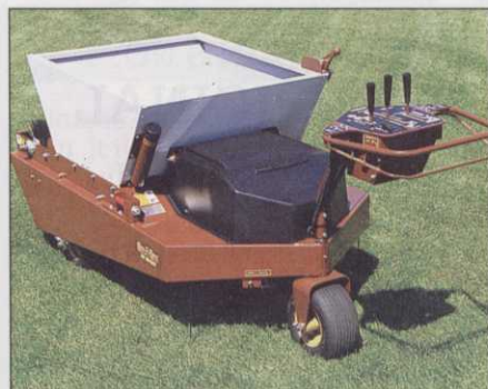
Above: Turfco Mete-R-Matic self propelled top dresser from Turf Machinery Ltd has a patented chevron belt conveyor for precise application of dry and damp materials at varying rates. Top: Able to carry up to 500kg of material, the Ultra Plant UP30 top dresser has a serrated roller and brush feed mechanism.
