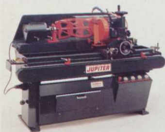
42" capacity Mower Cylinder and Bottom Blade Grinding Machine. A truly 'precision' grinder, built to last half a century. Used and preferred by professionals.
