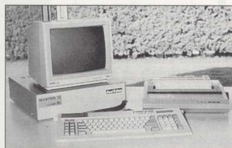
A Rainbird Master II multizone controller with printer Picture courtesy of Wright Rain Ltd
