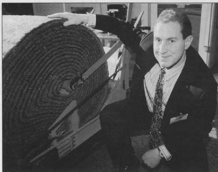
Simon Hannam, a technical adviser with the Inturf Group shows off the company's latest installation machine. The lightweight machine has a synchronised feed which places the turf precisely onto the rootzone irrespective of the forward speed of the machine. The TIM system is operated by Inturf's team of greenkeeping staff as an in-house service. Tel: 0759 304101
