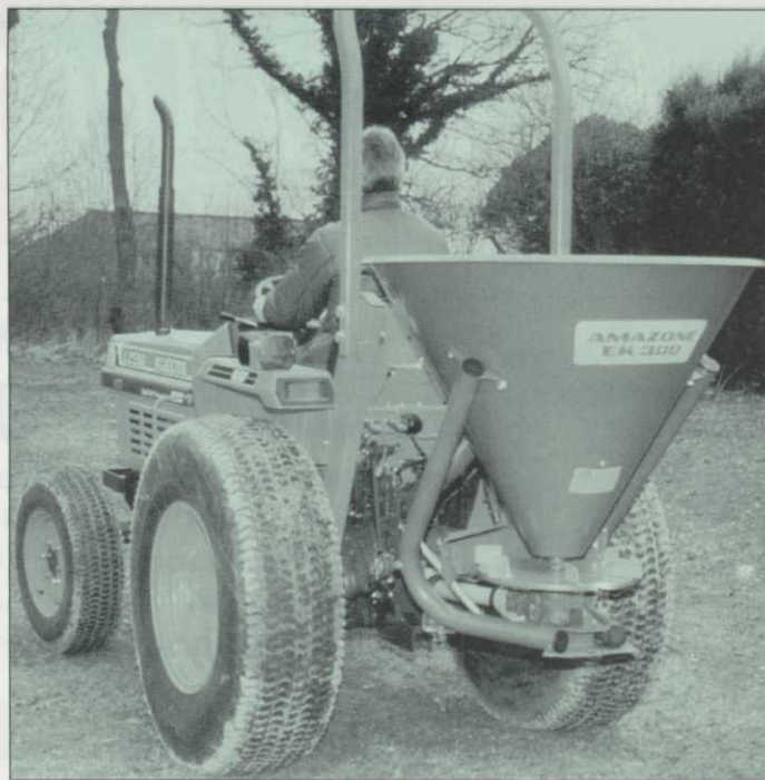
Amazone's EK 300 spreader is a single disc machine with a 300 litre hopper capacity and spread width from 3m to 12m depending on material. Ensure that the machine is set level and at the recommended working height.
