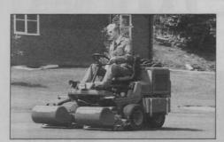
**Huxleys have introduced** a new version of the increasingly popular 358 Greensmower. Changes to the hydrostatic pump, reel drive pump and wheel motors have enabled the maximum engine speed to be reduced to 2100 rpm. This provides extremely quiet operation, reduced fuel consumption, less wear on engine and transmission and a smoother, cooler and more simple operation.
