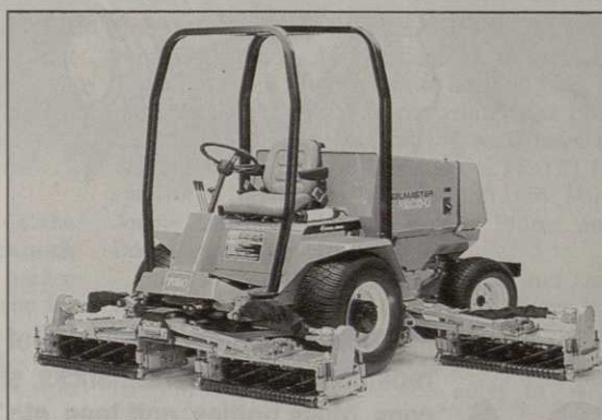
A roll-over protection structure, four-wheel drive and improved cooling system are key features of Toro's Reelmaster 4500-D
