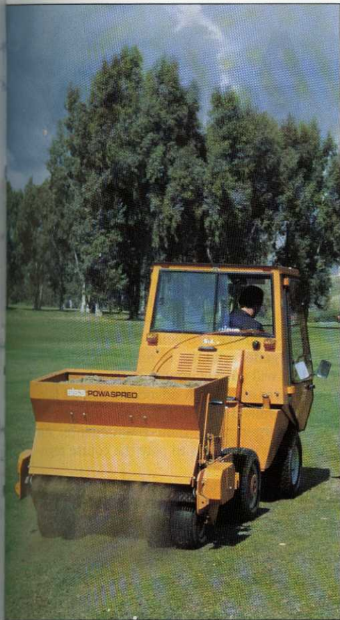
Built to apply a variety of top dressings across a 48in (1.22m) width, the pto driven Sisis Powaspred is available in trailed and fully-mounted versions to suit a wide range of power units. Delivery from the 14cu ft (396 litre) hopper is by rotating brush and output is 2 acres/hour at a forward speed of 4mph. A 78in (1.98m) model is also available
