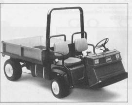
The transaxle features three speed syncromesh gears for easy shift and quiet operation, plus a hi-low range for six distinct working speeds, and manual differential lock. Also featured is a third gear supervisors lock-out, which reduces the maximum speed from 23 to 13.6 mph.
