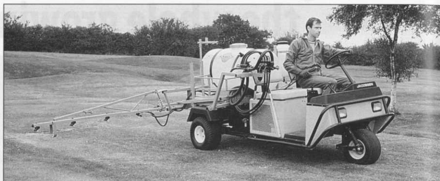
Hardi AM-PS de-mountable sprayer on a Jacobsen Workhorse
