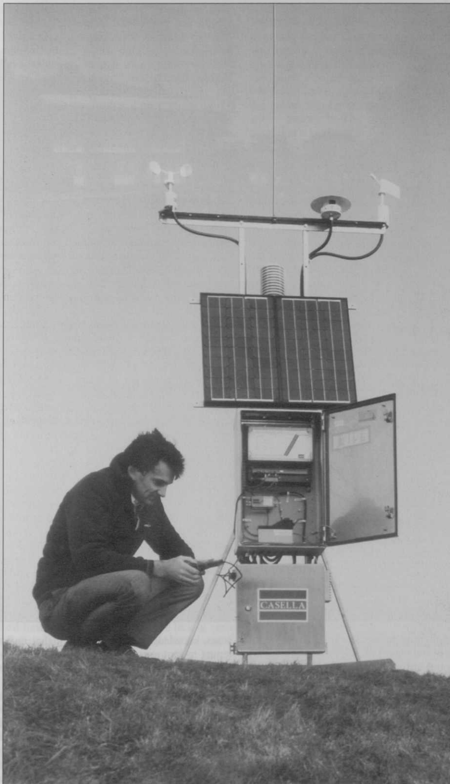
A somewhat sophisticated weather station, the Intelligent Automatic Station by Casella
