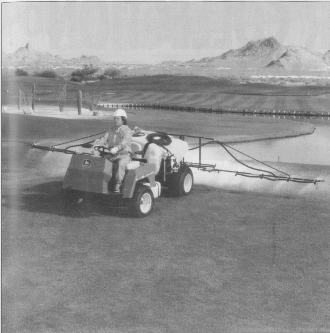
A forward driving position provides an excellent view over the work while enhancing the balance of the machine, especially when using rear-mounted attachments
