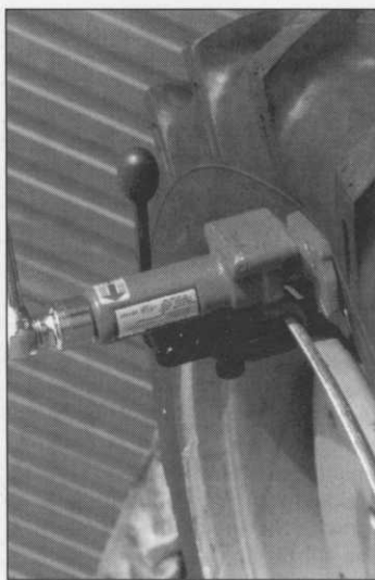
Up to 10 tonnes of pressure is produced by the Bead Buster to help remove tyres from rims without the use of hydraulics, pneumatics or very large sledge hammers
