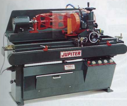
42" capacity Mower Cylinder and Bottom Blade Grinding Machine. A truly 'precision' grinder, built to last half a century. Used and preferred by Professionals.
