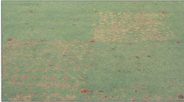
2. STRI field trial evaluating oil/hydraulic fluids for adverse effects on fine turf
