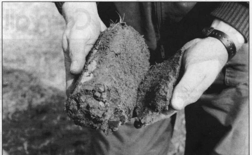
Core sample showing ProBase 3 inserted by Cambridge Sand Groover
