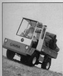
■ Spanish manufacturer, Ausa, has introduced MULTITRANS DV17, a 1500kg payload utility vehicle. Powered by a water cooled 21.7hp Isuzu diesel, DV17 features 4 forward and 4 reverse gears and has a top speed of 16mph. Power to weight ratio is impressive and there is plenty of power in reserve for towing trailers.
