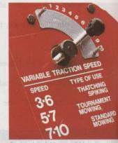
Optional variable speed kit ensures precision cutting by allowing the operator to select a consistent ground speed while maintaining a constant, even clip. This another course of action which be instrumental in changing the pattern of wear.
