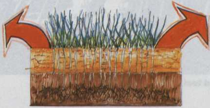
Air channels are closed; the air is forced out and water can no longer move freely in the soil
