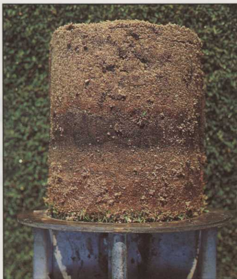
A black layer in a pure sand green. This layer has developed because conditions in the green are anaerobic for long periods, due to inappropriate choice of sand and deficiencies in maintenance. This is formed by metallic sulphides (e.g. iron sulphide) which are created under intensely anaerobic conditions by sulphur-reducing bacteria. These intense anaerobic conditions are sufficient to kill turfgrass roots
