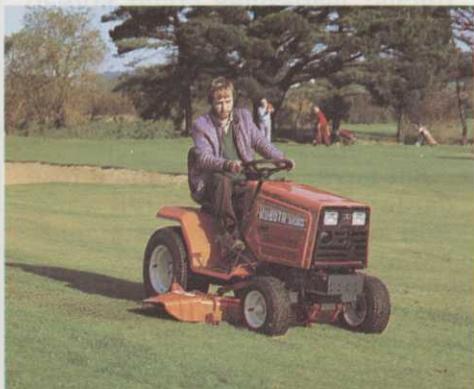
G3HST—with hydrostatic transmission and 44" mid-mounted mower, that makes short work of light rough. Highly manoeuvrable, with miserly fuel consumption and minimal maintenance.
