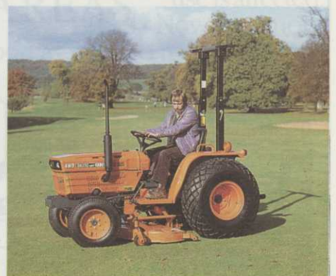
B8200—with a 3 cylinder, 19hp engine (and the option of hydrostatic transmission), this is the perfect machine for heavy duty work.
