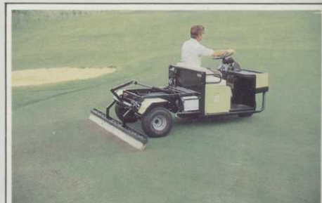
GREENS BRUSH (H33): For general use on sports turf, the switching of golf greens and effective brushing-in of top-dressings, the Huxley 8ft Greens Brush has a spring-loaded frame to follow ground contours. It can be raised and lowered hydraulically from the driver's seat providing precise control over operating height and degree of brushing action, as well as affording convenient movement from site to site.
