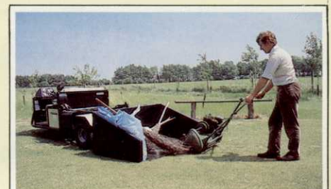
LOW-LOADING TRANSPORT CARRIER (H32): Fully mounted on three pins at the rear of the Turf-Truckster, the robust Transport Carrier combines a handy ground level loading ability with a useful carrying capacity for general maintenance tools and materials. Internal dimensions are 60in wide x 36in deep. The complete unit is raised and lowered using the Truckster's hydraulic system, controlled from the driver's seat.
