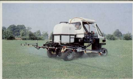
SPRAYER (H6): Mounted directly onto the Turf-Truckster's chassis, the 66 gallon (300 litre) Huxley sprayer has a three-section, 19½ft (6m) boom, pto-driven diaphragm pump and colour-coded nozzles. Application rate range meets all turf spraying requirements. Operating controls are grouped conveniently to the driver's right hand and a high pressure hand lance with 50ft of hose are standard.
