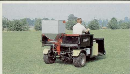
CYCLONE SPREADER (C3): Designed to spread fertiliser and seeds across swath widths of up to 40ft, the Cushman Cyclone Spreader has a 300lb capacity and is driven, by flexible shaft, direct from the Truckster's pto. The spreader has a galvanised steel hopper and attaches quickly onto the rear of the H5 Short Dump Box or H7 Longbox. Rotary agitation prevents bridging of materials and output is varied by sliding gate.
