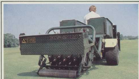
GREENSAVER AERATOR (C10): The Cushman Greensaver Aerator, with Weight Box set, is able to perform virtually all hollow coring (with core collection) and shallow aeration operations on fine turf. Three drum types are offered: standard \frac{1}{2} in coring drum (shown here), with trap door for rapid core disposal; \frac{3}{8} in coring drum, with trap door; and 2 \frac{1}{2} in deep slicing drum. All produce a 3 \frac{1}{4} in x 4in aeration pattern.
