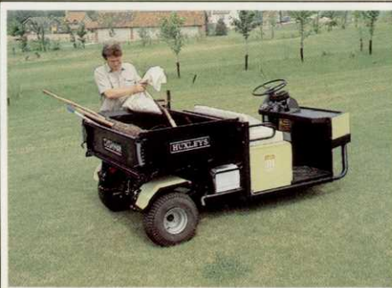
SHORT DUMP BOX (H5): With its 1,500lb payload, the rugged Huxley Short Box is ideal for handling loose and bulky materials as well as small machines and hand tools. Both hydraulic tipping and tailgate release are controlled from the operator's seat. The unit measures 35in x 52in x 12in internally and it attaches to the Cushman Turf-Truckster using just three pins – please see back page for detail of tipping ram and connecting pins.
