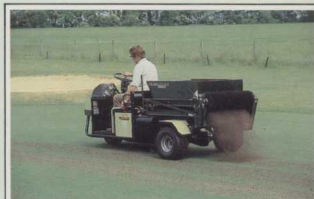
TOP DRESSER (C5): Mounted on the Turf-Truckster's chassis and driven by the power take-off, the Cushman Top Dresser produces a precise and even spread of most free-flowing materials across a 31 \frac{1}{2} in width. Capacity is 9 \frac{1}{2} cu ft (approx. 1000lbs) and delivery is by a combination of belt conveyor and rotating nylon brush. Application rate is controlled by metering gate, with drive engaged/disengaged from the driver's seat.
