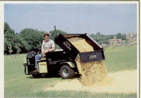
SHORT DUMP BOX (H5): With its 1,500lb payload, the rugged Huxley Short Box is ideal for handling loose and bulky materials as well as small machines and hand tools. Both hydraulic tipping and tailgate release are controlled from the operator's seat. The unit measures 35in x 52in x 12in internally and it attaches to the Cushman Turf-Truckster using just three pins – please see back page for detail of tipping ram and connecting pins.
