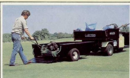
TURF TRAILER (H40): This low-loading work trailer, with its 1,000lb (approx. 23 cu ft) capacity, was developed by Huxleys for use with Turf-Trucksters and other suitable vehicles. It has a clevis-type tow hitch, special wide turf tyres and a ramp tailgate for the convenient loading of a wide range of grounds maintenance equipment and materials. Internal dimensions are 58in x 42in x 16in.
