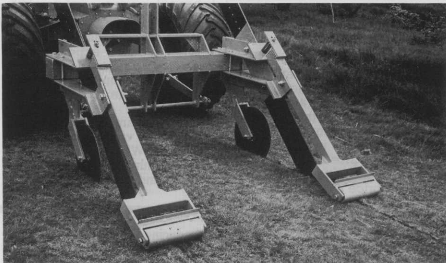
The SISIS Hydrotrac fitted with a double mole plough.
