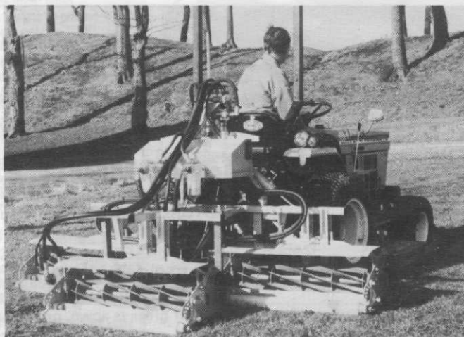
The Green's Bantam triple hydraulic cylinder mower.
